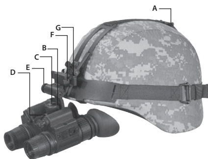
FIGURE 3-3. MOUNTING THE N-15 TO A HELMET
