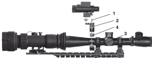
FIGURE 2-5. PLATFORM RING INSTALLATION
