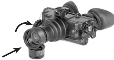
FIGURE 3-4. INSTALLATION OF COMPASS
