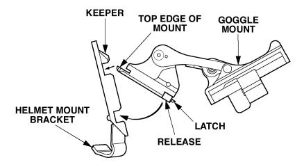
Figure 2-4. Installation of Helmet Mount.
