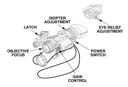
Figure 1-4. Mechanical Functions of the MNVD.
