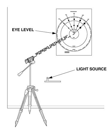
Figure 3-7. Dark Room Setup with Tripod.
