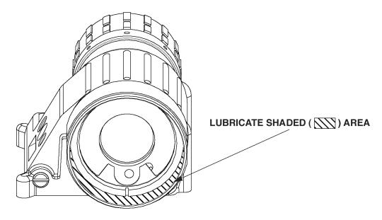
Figure 3-14. Applying Lubricant to Inside of Monocular Housing.
