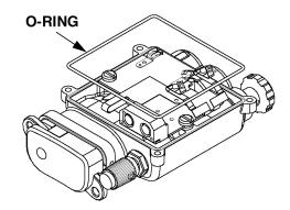
Figure 3-19. Installing O-Ring.
