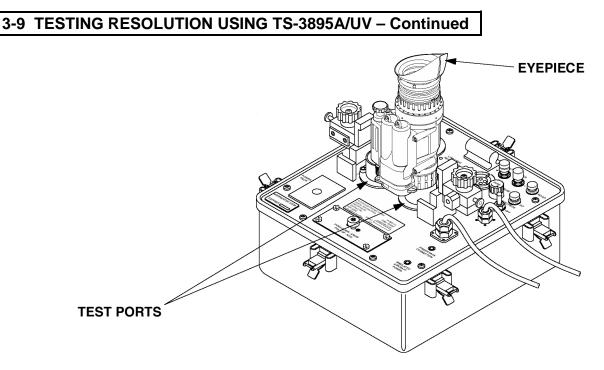
Figure 3-2. Inserting Monocular into Test Set.
