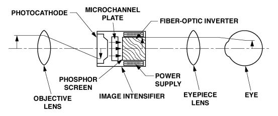
Figure 1-5. MNVD Optical Function Diagram.
