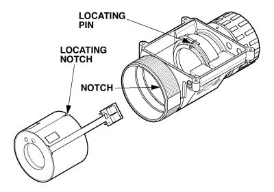
Figure 3-23. Inserting Tube into Monocular Housing.
