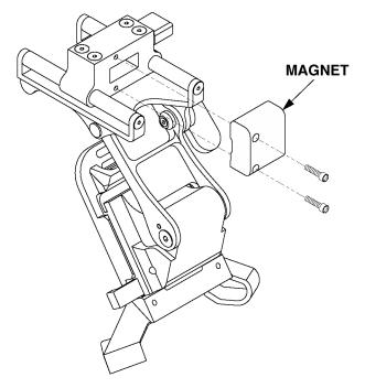
Figure 2-5. Magnet, Metal Helmet Mount.
