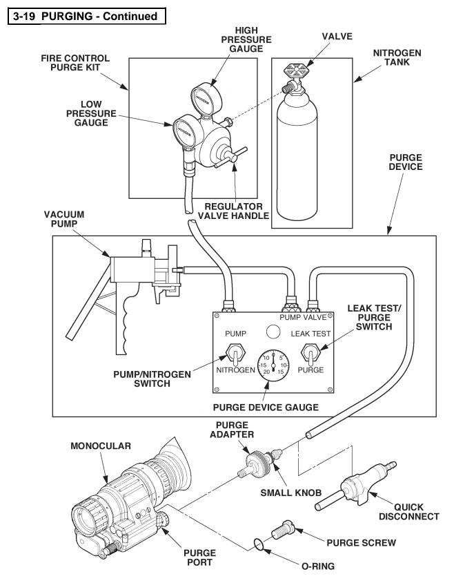
Figure 3-29. Nitrogen Purging Equipment Setup.
