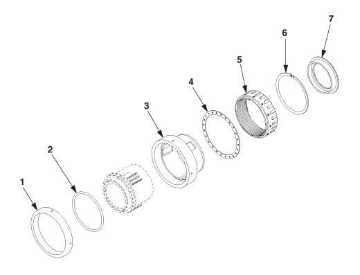
Figure C-3. Eyepiece Assembly.
