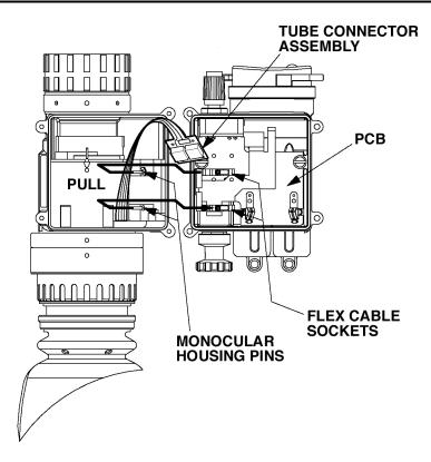
Figure 3-18. Battery Housing Connections.
