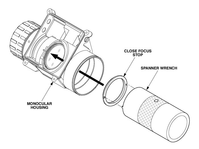
Figure 3-27. Installation of Close Focus Stop.
