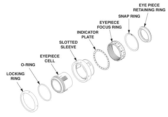
Figure 3-10. Components of Eyepiece Lens.
