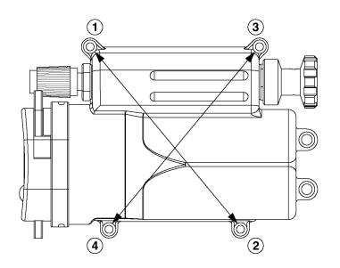
Figure 3-21. Tightening Screws.
