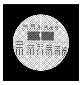
Figure 3-17. Properly Focused Diopter Image Using TS-3895A/UV.
