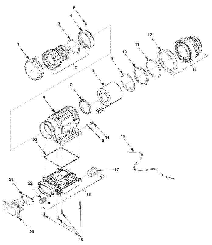
Figure C-2. Monocular Assembly, AN/PVS-14.
