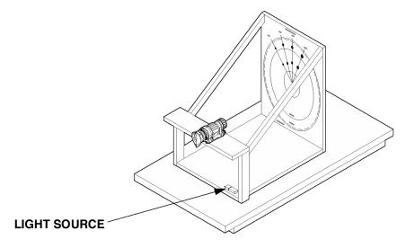
Figure 3-6. Dark Room Setup with Test Fixture.
