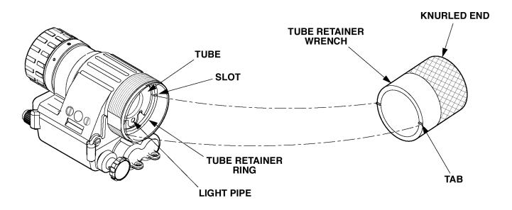
Figure 3-22. Removal of Tube Retainer.
