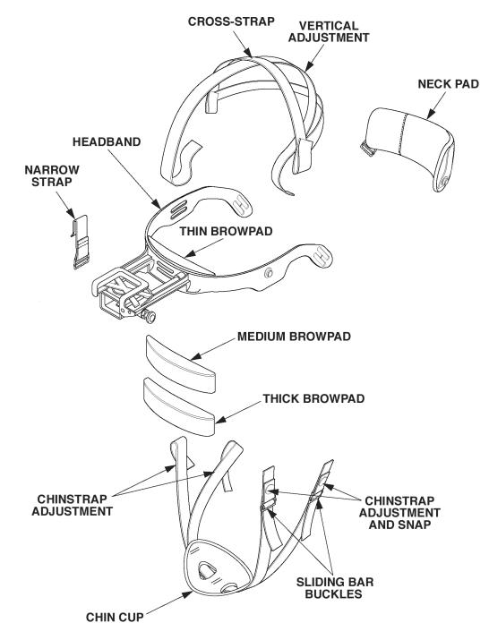
Figure 2-1. Headmount Components Removal and Installation.
