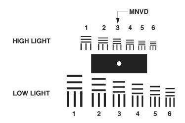
Figure 3-4. High Light Element In Resolution Test Pattern.
