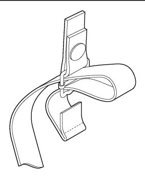
Figure 2-3. Lacing of Sliding Bar Buckles.
