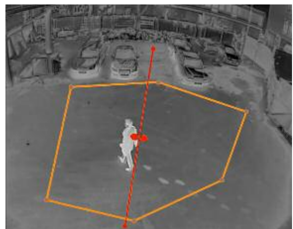
Easily configure designated borderlines and secure zones simply by drawing lines.
